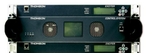
Passive Reserve configuration with control system
