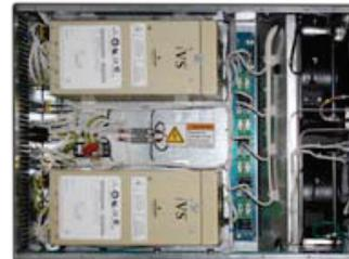
All high power amplifier stages use parallel transistors to ensure excellent availability. This simple design enhances reliability by reducing component parts count and minimizing harnessing and single point paths, resulting in high MTBF performance. At the same time, the simplicity of the design eases installation and maintenance.
